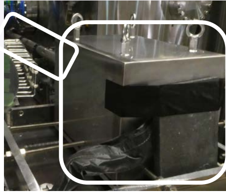
HX detector with long heavy -alloy collimator
