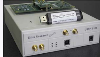
SDR for ECE heterodyne radiometer
