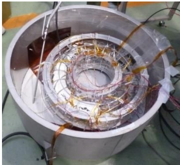
Short sample (~3 m) test Bent radius :1-0.2 m @77 K, 0 T
