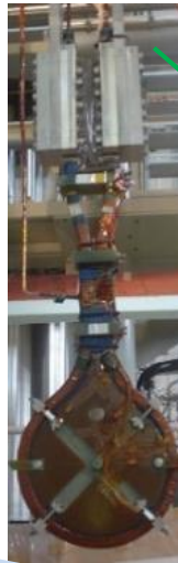
Short sample (~3 m) test Coiled ( \phi 0.5 m) @20 K, 9 T
