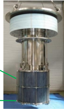
Short sample (>3 m) test Coiled ( \phi 0.6 m) @20 K, 13 T
