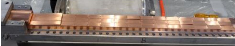
Bridge-type mechanical lap joint “Invisible joint”
