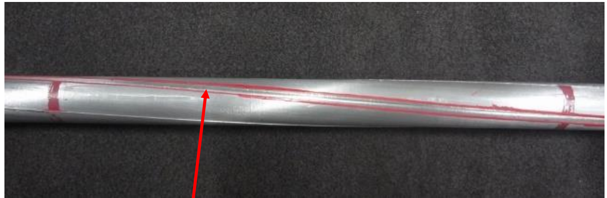
Twist pitch: 2 rotations / m
