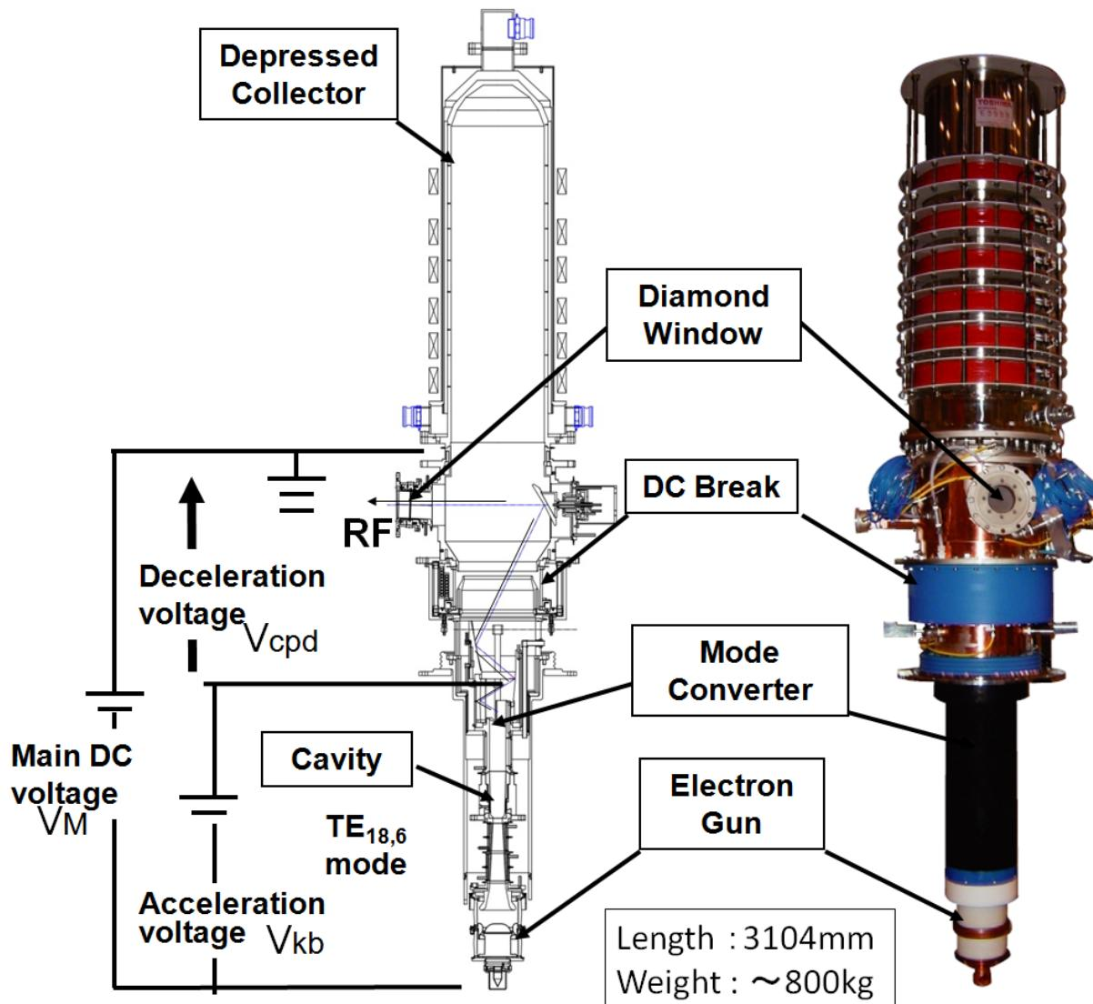
28 GHz gyrotron has been developed for Gamma-PDX projects at Tsukuba University by themselves.
