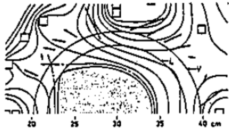
Fig. 2. An example of poloidal-field measurements for the case of D-shaped cross section. The values of the current
